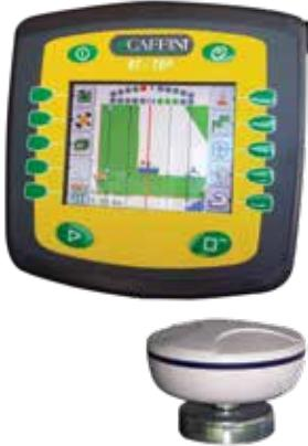
**Computer: IsoBus:** Modern computers enable the fully automatic control of the application. A large coloured back-lit screen guides through the easy to manage and control menus.
