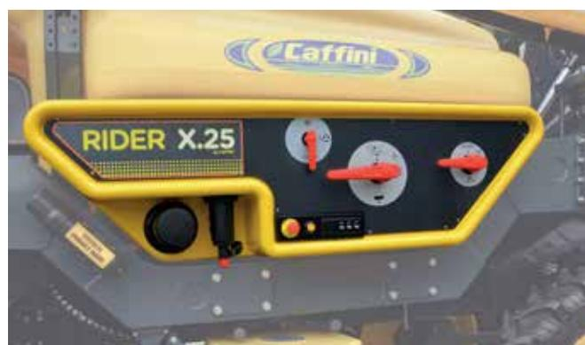
**Hub Service:** work station for preparation of spraying treatments. All operations can be carried out in the same place thanks to multi-purpose valves for: checking of the loading, return, system and tank washing phases. Their activation is guided by coloured pictograms.
